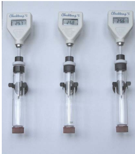
Experimental design to measure the absorption of heat by different gases (air, methane, CO 2 )
