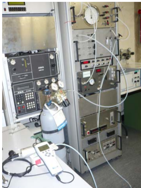
calibration of Vaisala sensors in the laboratory at Mannheim Hochschule
