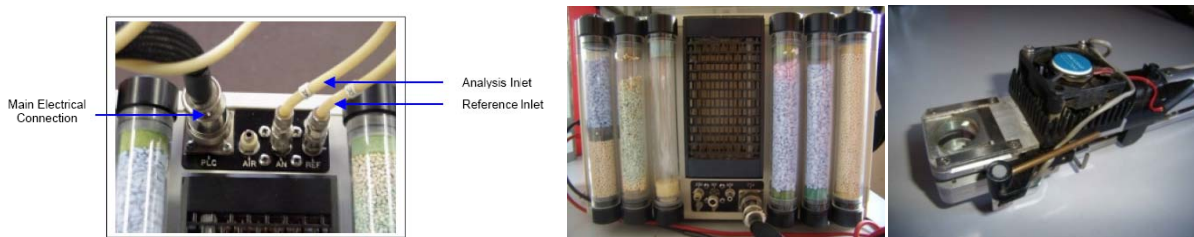
Fig. 1 CIRAS-1 Portable Photosynthesis System is made by three the Portable IRG and bythe Leaf Cuvette.
